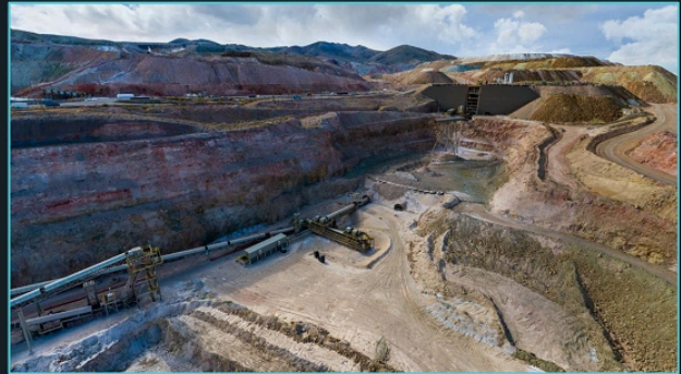
CRUSHER AND CONVEYOR BELT CIRCUIT
